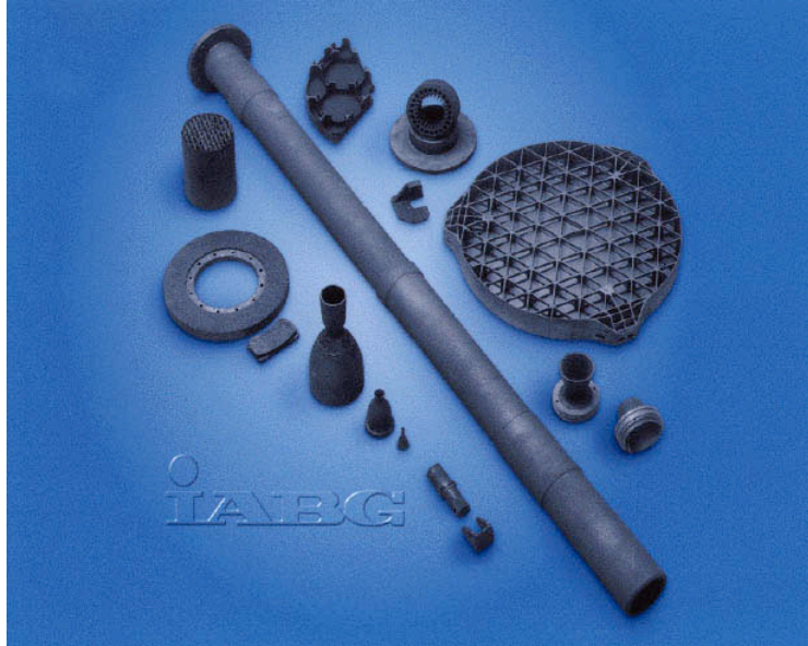
Fig. 2 Typical C/C-SiC parts (disc brakes, rocket nozzles, telescope mirrors, etc.) fabricated by the LSI process using random oriented chopped C/C felt (BPM/IABG).
