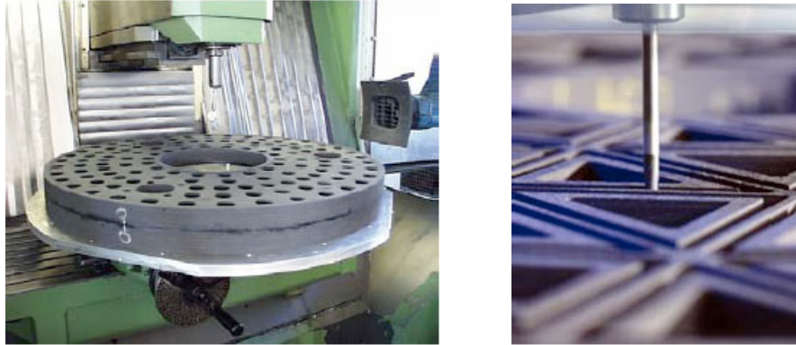
Fig. 7 Photos of numerically-controlled milling being performed on carbon-carbon green-body material [5].
