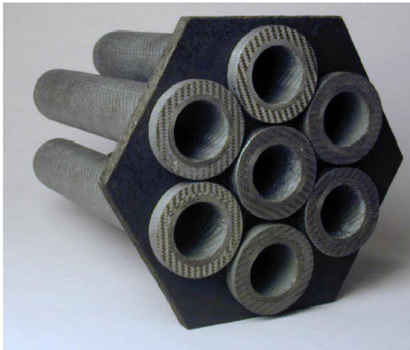
Fig. 4 LSI composite heat exchanger with 0.3-m long tubes being developed for high-temperature (950 – 1200°C) heat recovery from moist flue gas to indirect high-pressure gas power cycles under the EU HITHEX project [2].
