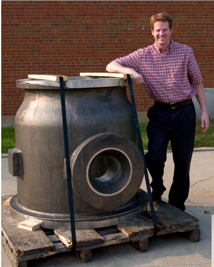
6,700 lb CF8C-Plus end-cover cast by MetalTek for Solar Turbines Mercury 50 gas turbine
