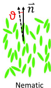
Figure 3.2: The angle \vartheta between the orientation of a molecule in respect to the director \vec{n} defines the order parameter S .
