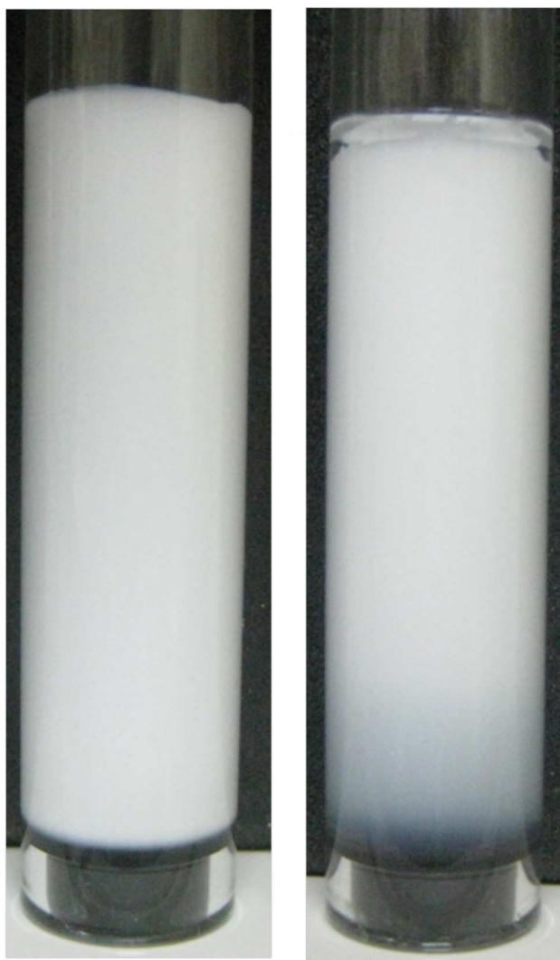
FIGURE 7.12 – Photos recorded for the C14/GuHCl/NaOH system at a concentration of 44 mM : sample tube just after emulsification (left) and for the same emulsion after six days (right).
