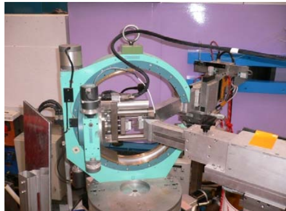
Fig. 1: experimental setup on G5.2 with the tensile machine mounted on Eulerian cradle.
